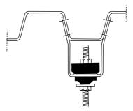
Square duct fastened to the ceiling with SAFID duct fixing bracket, air duct fasteners, threaded rods and steel anchors.
