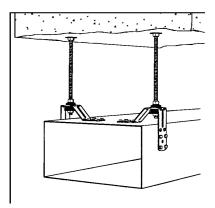
Sound insulated fastening of a SAFID support channel profile on a metal sheet with wide trapezoid corrugations using SAFID duct fixing bracket.
