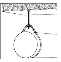
Direct fastening to a metal sheet with trapezoid corrugations using SAFID duct fixing braket.
